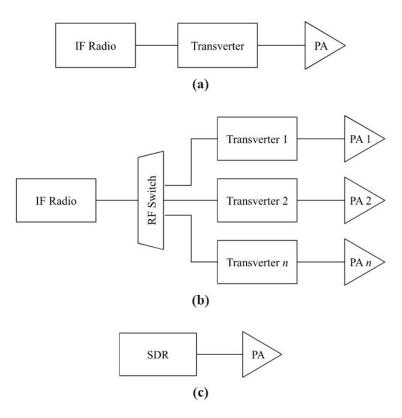
Figure II. Microwave Radio Architectures (a) Transverter (b) Transverter, Multiple Bands (c) SDR
