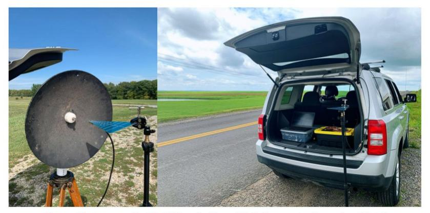
Figure V. Antenna for Field Test (left) and Full System in Operation (right)
